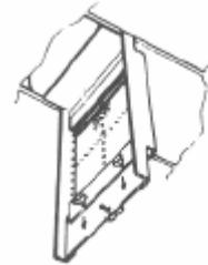
8. Insert hinge pins of the prismatic lens into the slotted receptacle located at the bottom rear corner of the housing. Raise the prismatic lens to the horizontal position and secure it by pushing the 2 – slide mounted fasteners to take their extended position.
