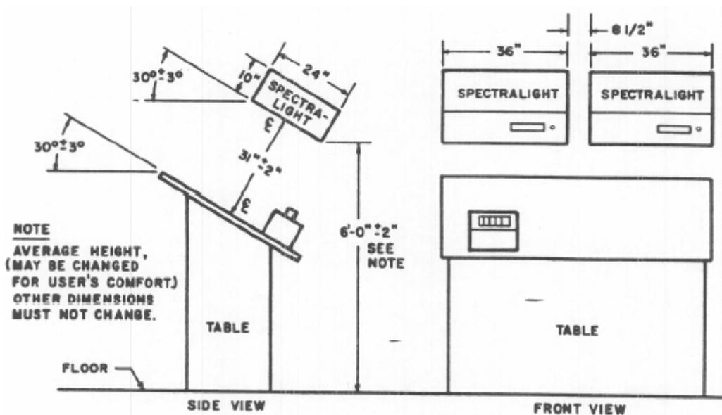
Dual instrument suspended installation
